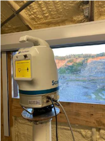
Fig 1. The laser scanner operating from within the synchronized protective field enclosure.
